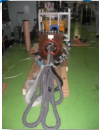
20kA/200kVA Transformer for heavy current test
