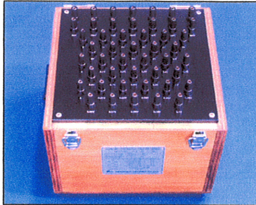
AUXILIARY VOLTAGE TRANSFORMER
