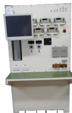
ANF-10 (P) Control board for ELCB test
