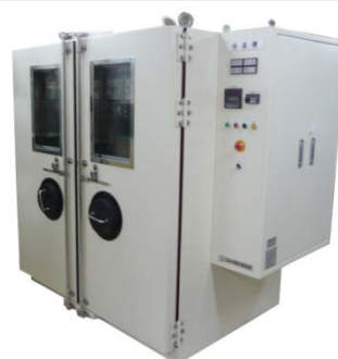
ANF-10 (B) For ELCB temperature test (Available for inclined test with remote controller)
